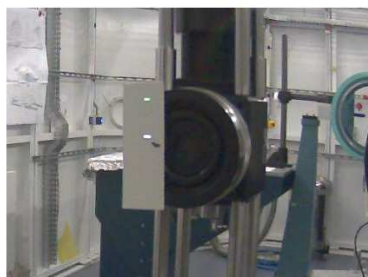
Direct beam and reflected beam by KB mirrors at sample position
